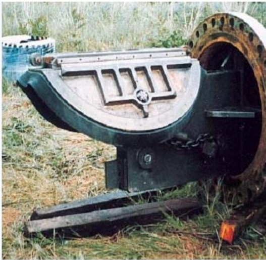
FOLDING HEAD SYSTEM Sequence of 36" (ND 900mm) folding head installed in steel cylinder reinforced concrete test pipe
