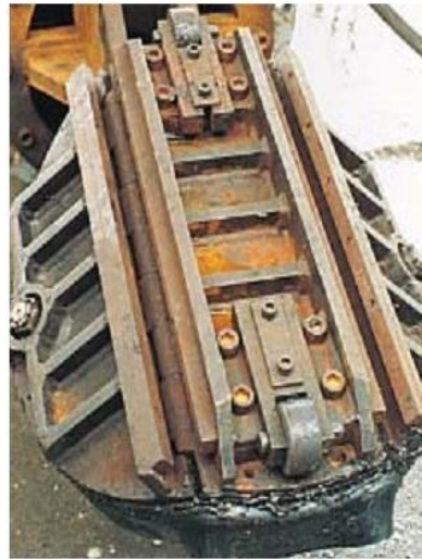
FOLDING HEAD SYSTEM Sequence of 36" (ND 900mm) folding head installed in steel cylinder reinforced concrete test pipe
